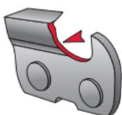
Severe abrasive damage on side plates.
