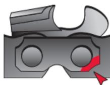
Peening on front corners of cutters and tie straps.
