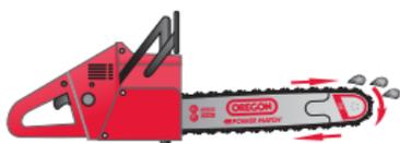
5. ▲ ■ Saw chain tension is especially important when the chain saw is tipped on its side during felling cuts. Loose saw chain (and rim-type drive sprocket, if used), will slide down and out of alignment with the guide bar. Loose saw chain tension is the leading cause of drive sprocket problems.
