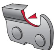
Light abrasive damage on side plates.
