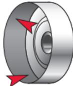
Excessive wear on the inside surface of the drum skirt.
