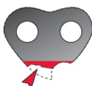
Battered and broken bottoms.
