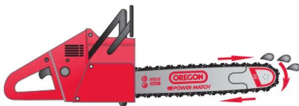
A constant supply of oil to your chain saw's guide bar, saw chain and drive sprocket is vital. Without it, excessive friction, wear, and damage will occur.
