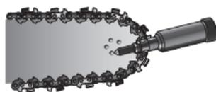
**NOTE:** Select a new nose sprocket with the correct pitch for your guide bar and saw chain.
