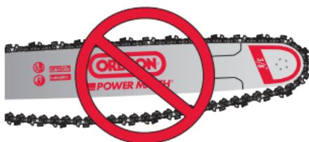
More saw chain and guide bar problems are caused by incorrect saw chain tension than by any other single factor. See pages 35 – 37 on how to tension your saw chain.
