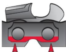
Peening on bottoms of cutters and tie straps.
