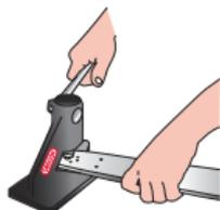
2. Use a small screwdriver to spread the guide bar nose rails just enough to remove the old nose sprocket. Clean out debris from the sprocket area.
