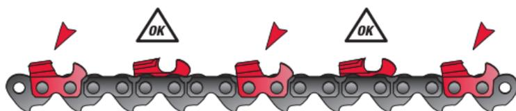
Damage to cutters on one side of the saw chain. Remedy: **See S.**
