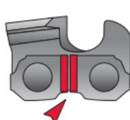
Tie straps between cutters, broken in the center.
