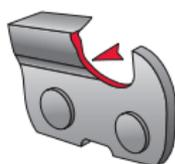
Abrasive or impact damage to the top plate or working corner.
